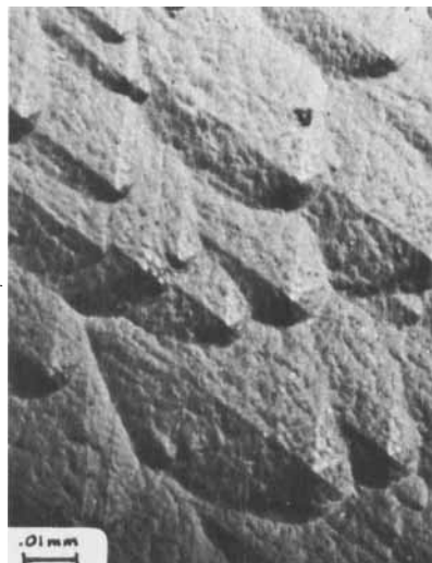
Figure 7. The appearance of the nearly hexagonal etch pits frequently observed on replicas of ice surfaces separated from solid substrates.
